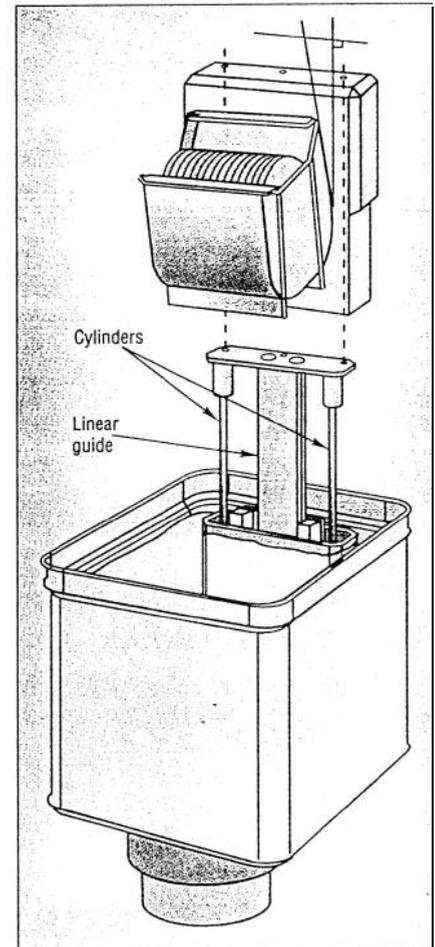
Water-powered cylinders stroke 14-lb elevator assembly with cassettes of silicon wafers into deionized-water rinsing bath. Cassettes are tilted 4° to keep wafers registered to left side.
