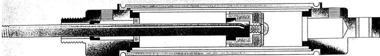
Carbon/graphite piston in Airpel cylinder floats on air, with no elastomer seals; 304 stainless-steel outer tube over Pyrex glass barrel provides impact protection. Modified version for water actuation at R Howard Strasbaugh is fitted with stainless-steel cylinder heads and piston/rod coupling also.
